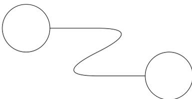
A spline is used in the same way as a line. When drawn continuously using `then`, a spline that changes direction draws a curve. (Similarly, a line would produce an angle). We'll see more examples of spline later.
