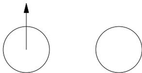
You can reference each type of object using an ordinal number. Referring to the order in which an object is drawn, you can say `first box` (1st box is also acceptable) or `2nd circle`. You can also work back from the last object, specifying the `last box` or `2nd last box`.
