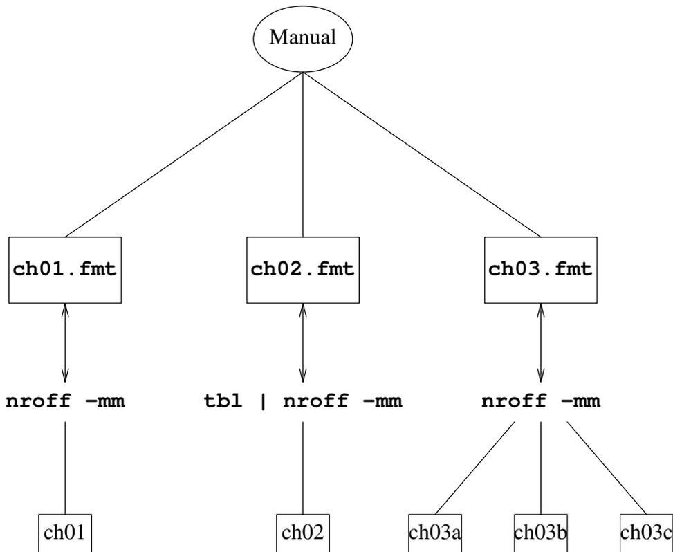
The target is `manual` and it is made up of three formatted files whose names appear after the colon. Each of these components has its own dependency line. For instance, `ch01 .fmt` is dependent upon a coded file named `ch01`. Underneath the dependency line is the command that generates `ch01 .fmt`. Each command line *must* begin with a tab.
