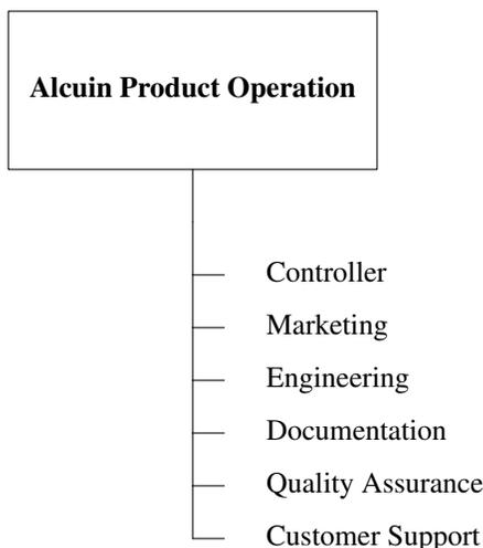
In the `pic` description that produced this drawing, the box is drawn explicitly and a short line is started down from the bottom of the box. Then a macro named `dept` is invoked to produce each item on the list.
