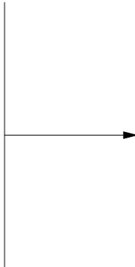
You cannot specify `down 1` or `right 1` without also specifying either a `line` or `move`. These attributes change the direction of the motion used to draw objects. They do not cause movement. The attributes of direction affect the position of the objects that follow it, as shown in the next example.
